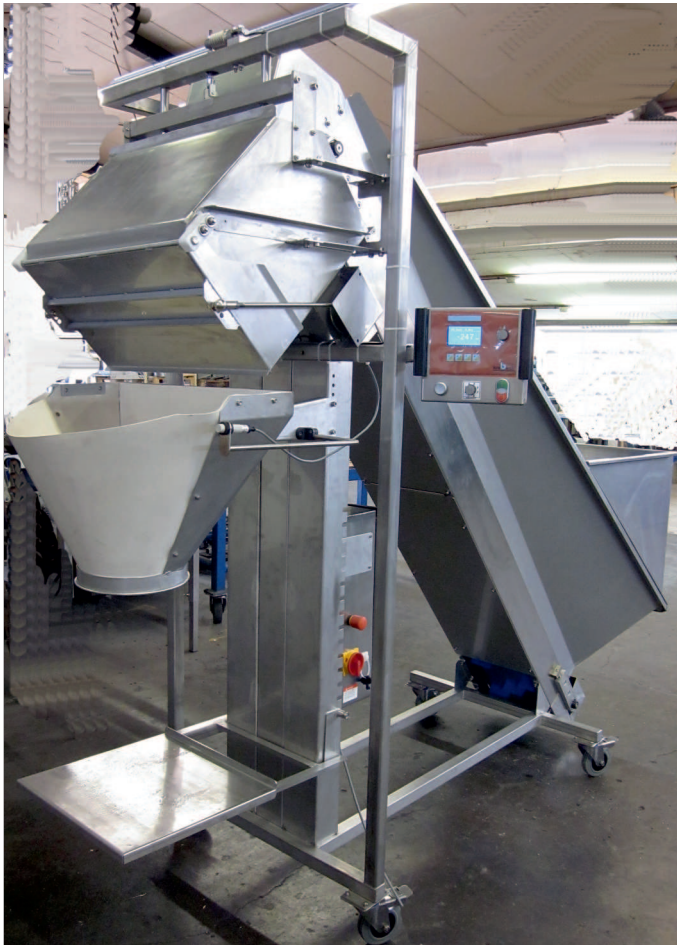
Bagging weigher KRD /3: suitable for potatoes, carrots, onions, charcoal and much more
